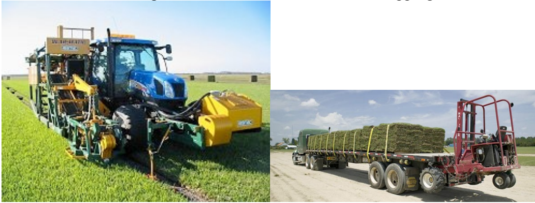
Sod Harvester and Sod Loaded on a truck for shipment
