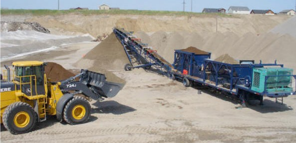
A Greensmix blender being loaded with Sand
